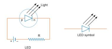
When p-n junction diode is forward biased, the electrons move from *n*-side to *p*-side and holes move from *p*-side to *n*-side. These charge carriers recombine near the junction and energy in the form of photons is released. The colour of light emitted by LED depends upon the band-gap energy.
