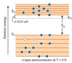
When *Ge* is doped with a pentavalent impurity Sb, *an n*-type extrinsic semiconductor is obtained and electrons are the majority charge carriers in it.
